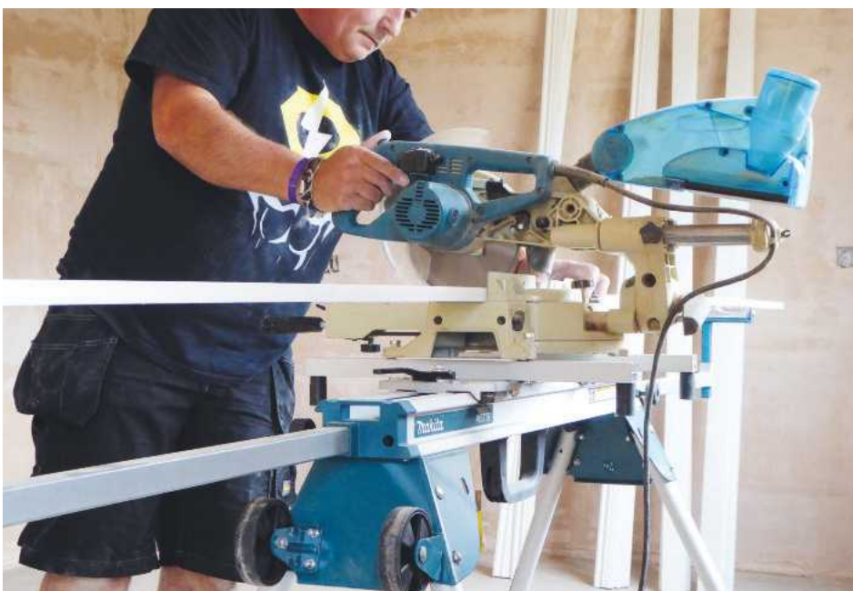
▲ Longer lengths of skirting and architraves are really easy to cut using the stand
